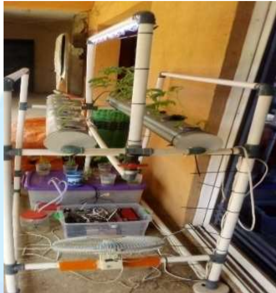
Figure2: Nutrient Film Technique Hydroponics Testbed with fourteen units of Tomato, Lettuce, Pepper and Spinach cultivated.
